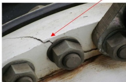
Fig. 8 Flange Brittle Failure
