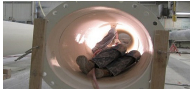
Fig. 5 Preparing to install an inside nozzle joint
