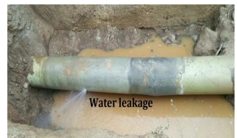
Fig. 2 Leaking Joints in a FRP pipeline the site due to defective manufacturing process, and usage of improper polymer/resin material and non-uniform sand content along with non-prescribed fiber
